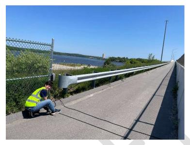
FIGURE 5 - 2023 SUMMER INTERN TROY IS SEEN INSTALLING TUBING FOR THE CYCLIST COUNT ON THE LITTLE BAY BRIDGE IN JUNE 2023. SOURCE: SRPC 2023.
